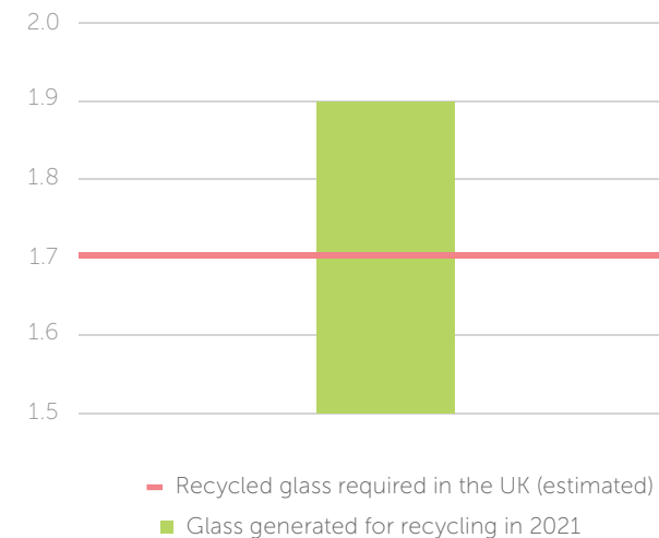
Quantity of glass required for recycling compared to the quantity of waste glass generated in the UK
